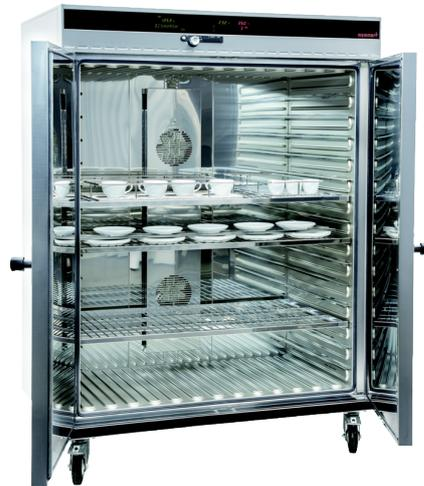
The Memmert heating oven dishwasher UFP800DW is specially adapted to the EN50242 standard and complies with the standard's specifications.
