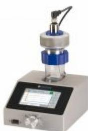
DPOT™ from GESERCO is a **water content analyzer** based on the "Aquatest" analytical technique which is standardized by ISO, AFNOR and GFC. Simple, fast and very precise, it is intended for use by maintenance departments, workshops and analysis laboratories for the monitoring of fresh and used fluids.
