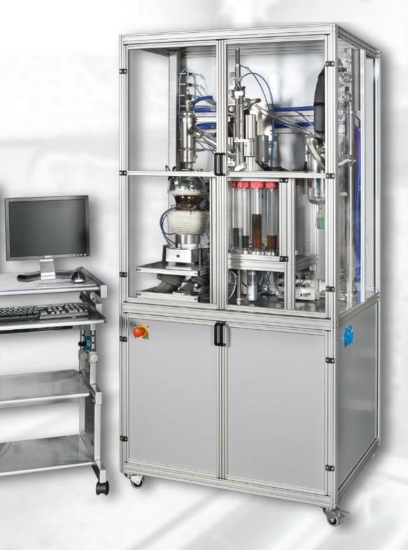
MPS and TBP-M have a carrousel, instead of a conveyor belt. The carrousel runs within a chamber, which has a front door. The chamber can be heated up to 90°C. It includes a volume follower system, cut weighing equipment and bottle closing.
