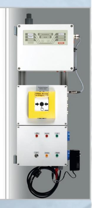
The fire extinguishing system consists of an infrared fire and smoke sensor, a detector electronic housing, it's own UPS box with charging unit and backup battery, an electromechanical trigger device and a bottle with Argon or Nitrogen.
