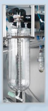
The water removal system is available as an accessory for TBP and Combi plants. It consists of a double mantle glass vessel (collector vessel) with internal quench cooler and bottom drain valve. The vessel can be removed when not in use. The collector vessel can be charged with 5 litre water/distillate mixture.
