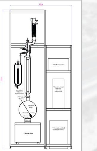
Alternatively, a stand alone water removal system is available. It comes with a complete framework with front doors, a complete set of glassware (condenser, reflux divider and column) and flask heater (with stirrer). The system comes with two thermostats; one for the condenser; one for the collector vessel.
