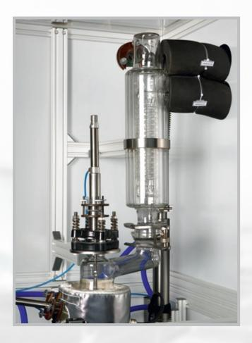
The high efficient triple mantle Condenser offers a large heat exchange surface, which exist of 2 separate internal coils and an external double mantle.
