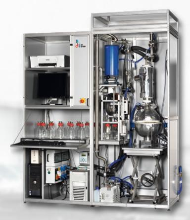
The ASTM D 5236 (Potstill) can fractionize crude oil or crude oil residue from  $15^{\circ}$ C up to 565 °C (at atmospheric equivalent temperature); from atmospheric pressure down to a vacuum of 0,1 Torr.
